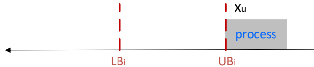
Figure 3-13. An activity node u starts and finishes after (UB_i) .
